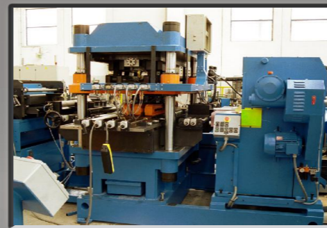
Detail of press and cutting shear
